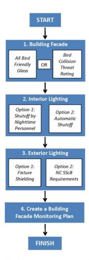
A building design that deters bird collisions will allow for most any type of site landscape design. Although the proximity and height of landscape material have shown to influence the number of bird collisions, if the building façade is designed to be "bird-friendly", the landscape material will not reflect and cause confusion to birds.
