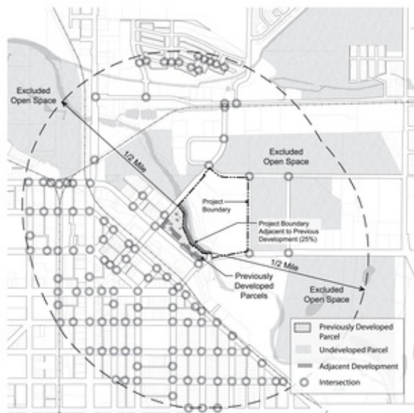
Figure 1. Adjacent and connected project site based on minimum 25% of perimeter adjacent to previously developed parcels and at least 90 eligible intersections per square mile (35 intersections/square kilometer) within 1/2 mile (800 meters) of boundary segment adjacent to previous development
