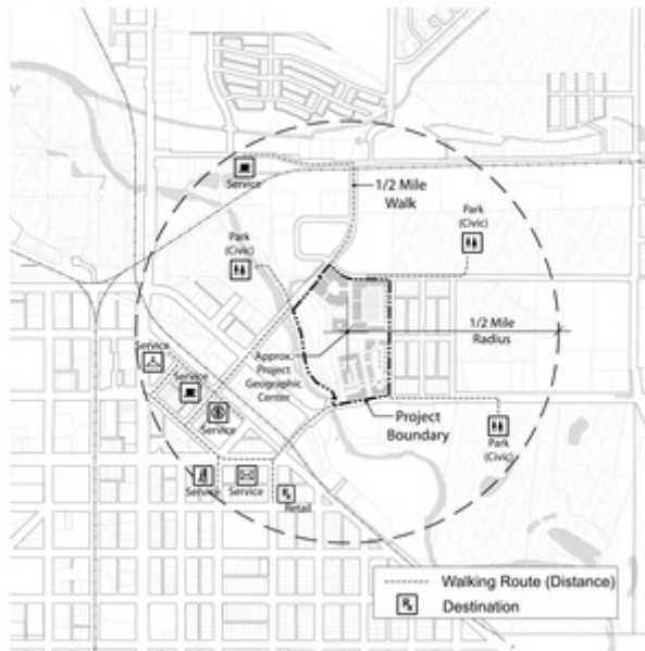
Figure 4. Walking routes on pedestrian network showing distances from dwellings and Nonresidential uses to transit stops
